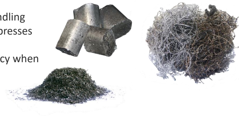
Pressing of the shredded swarf into handy briquettes.
