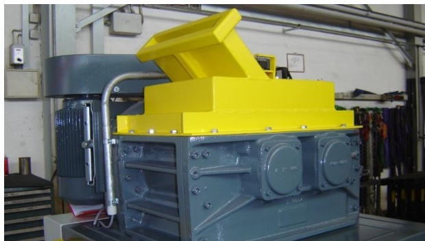
Hard disk shredder with special funnel
