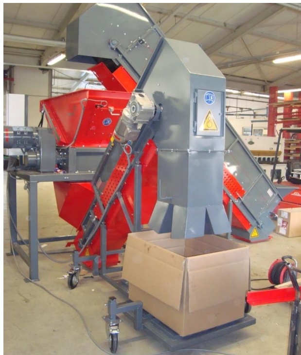
Shredding plant for landfills for material analysis
