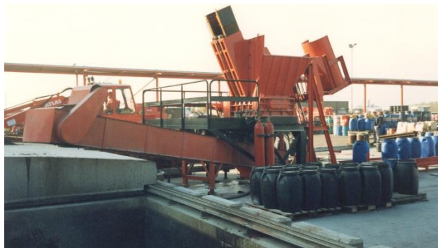
Shredding of PE drums in Germany
