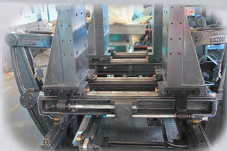
④中央支承模架 Central supporting frame for the mold
