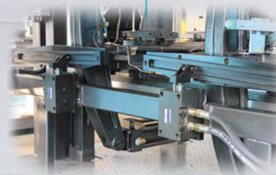
⑤移模速度控制阀 Speed control valves for mold's movement
