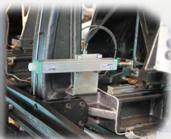
②电子尺控制开合模 Linear displacement transducer used to control the clamping units' movement
