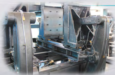
③平行式锁模 Parallel clamping units
